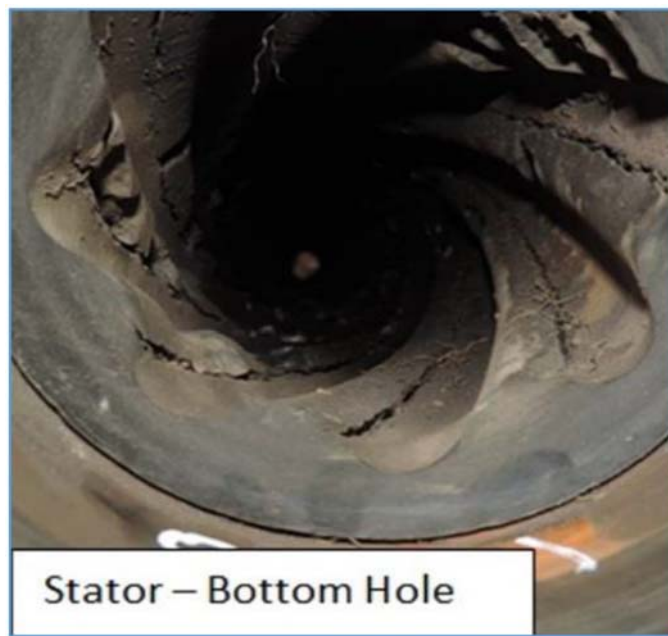
Figure 10—Example of failed stator due to fatigue.
